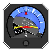
As bank angle and vertical speed approach the required amounts, bank angle and pitch-up attitude are shallowed. When the delta reference and the steering bars are matched the commands have been met. Thereafter, it is necessary to maneuver the aircraft to keep the display elements matched in order to accurately fly the programmed modes.
