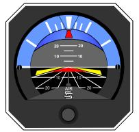
This system, which integrates both the roll axis and pitch axis, offers synchronized display of the flight profile. It is automatically activated when the autopilot is engaged. A Flight Director provides a visual indication of how accurately the pilot or autopilot is tracking the commands of the active mode of operation.
